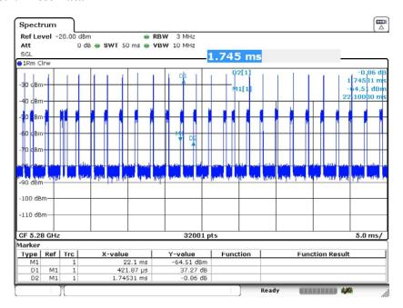
The resulting plot data was extracted and post processed, giving a duty cycle of 24.17%.
