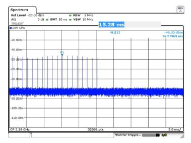
Peak of -46.33dBm, with losses at combiners factoring antenna gain to be 15.81dB, therefore level going into antenna port is -62.14dBm which exceeds threshold level of -64dBm for successful detection.
