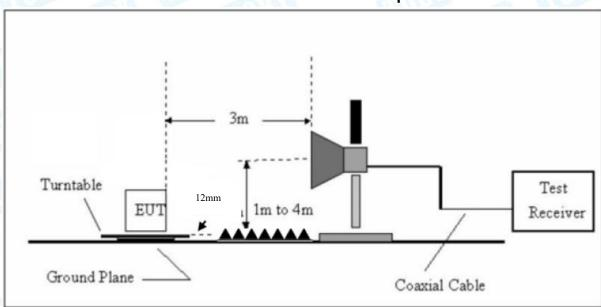
Above 1GHz Test Setup Conducted measurement
