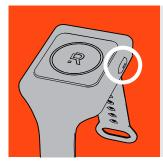
► If assembled correctly, the multi-function button should be visible through the small opening on the side of the wrist strap.
