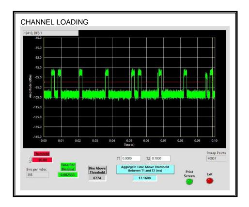
The level of traffic loading on the channel by the EUT is 17.16%
