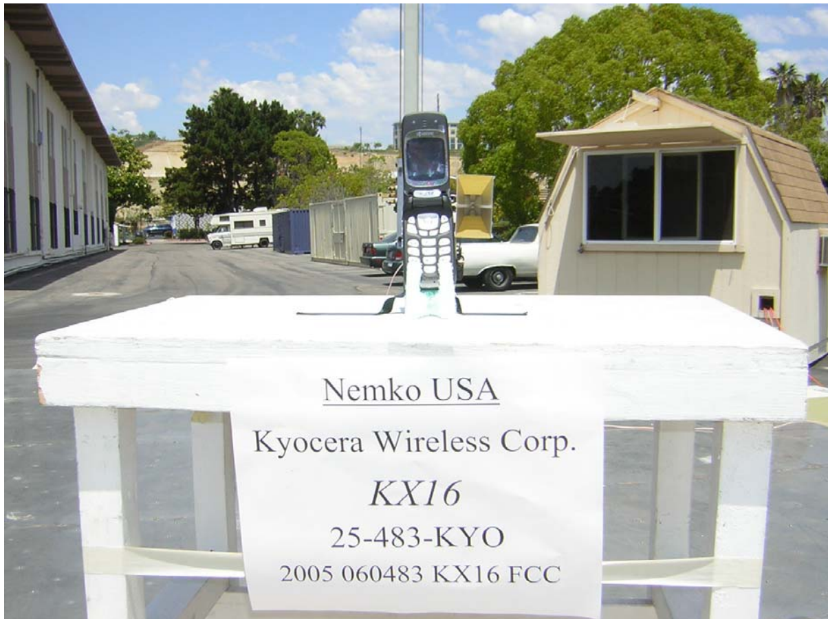
Photograph 3. FCC, Part 22/24 Radiated Emissions Test Configuration
