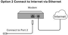
Note: To connect to the internet via another RJ45 WAN port (ports 3-6), configure your desired port to WAN, then connect the port to the internet via an RJ45 cable. Refer to FAQ-Q1 for more details.
