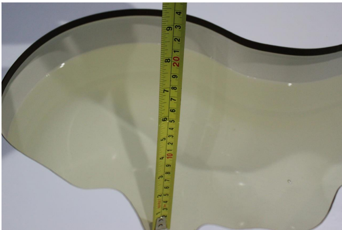
Picture 7-4 Liquid depth in the Head Phantom (5GHz)
