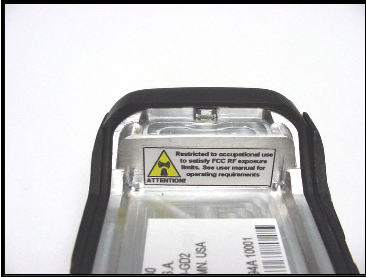
PHOTOGRAPH 2: RF LABEL AND LOCATION
