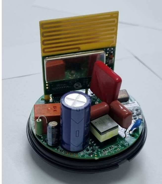
RF and Platform cards assembly
