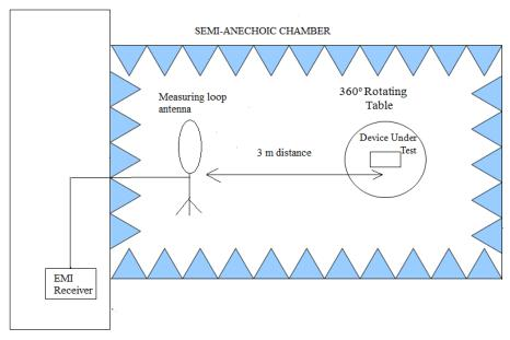
Shielded Control Room For Radiated Measurements
