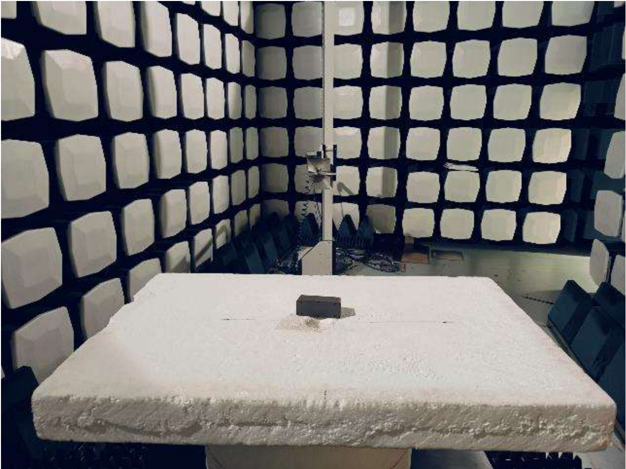
Picture 6 Radiated test setup, Back view, 1-18GHz
