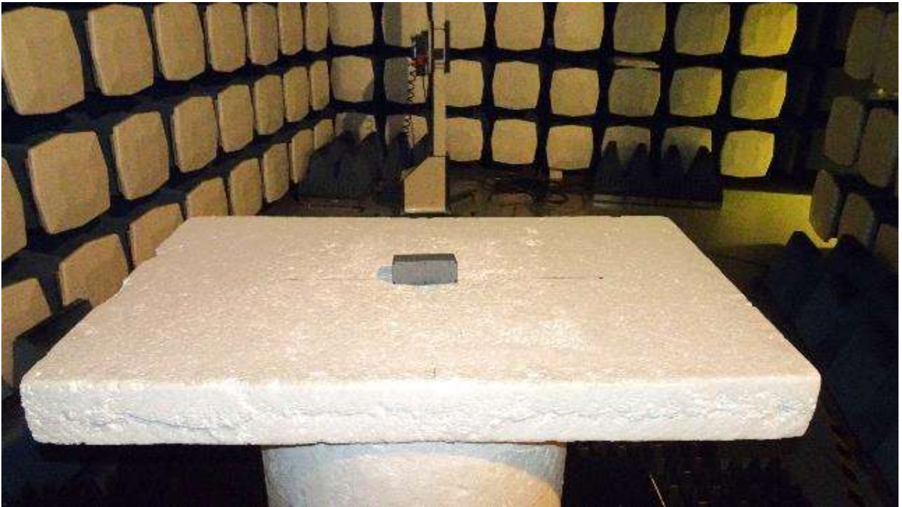
Picture 9 Radiated test setup, back view, 18 - 26GHz
