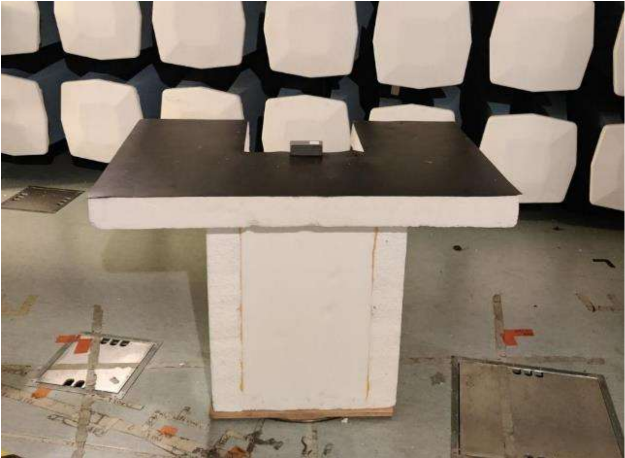
Picture 2 Radiated test setup, front view, 30 – 1000MHz
