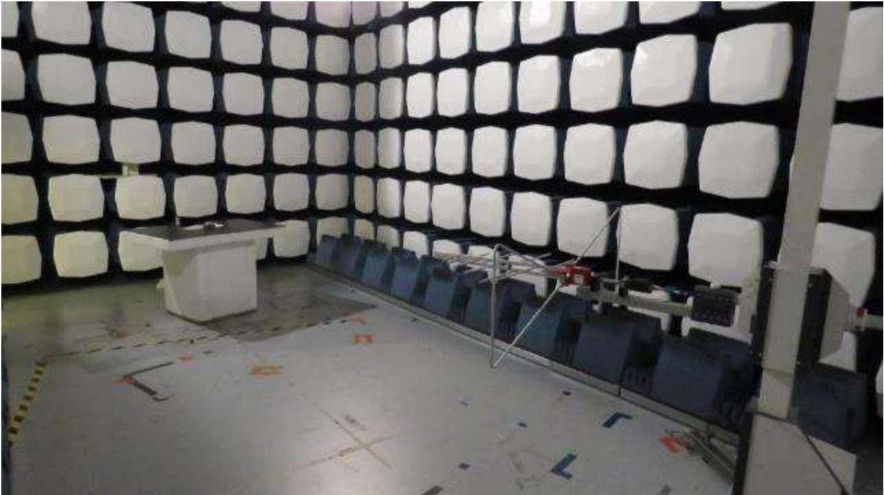
Picture 1 Radiated test setup, common view, 30 – 1000MHz
