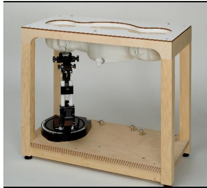
Picture C.8: SAM Twin Phantom
