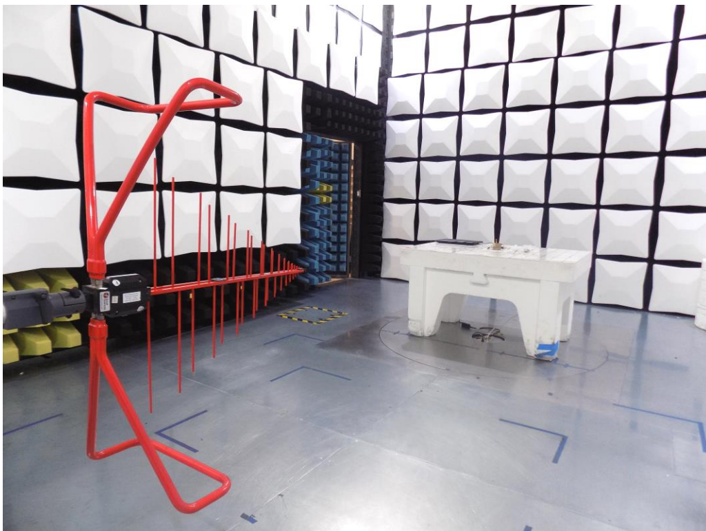
Figure 7 – Radiated Emissions 30 – 1000 MHz, Front View
