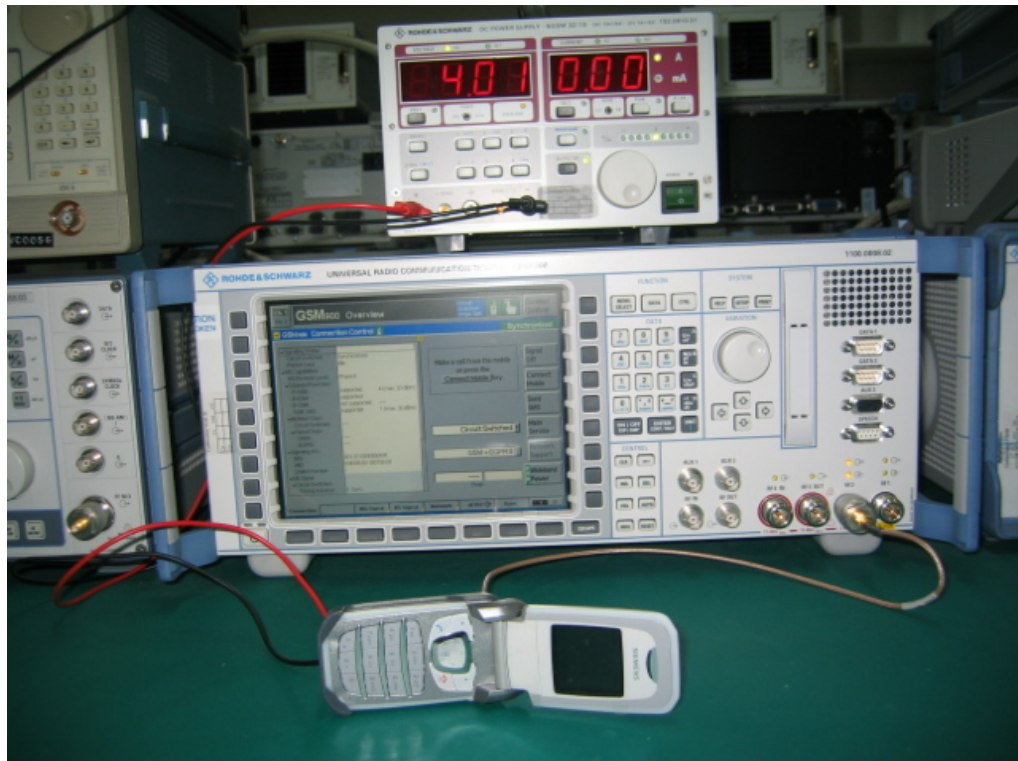
Figure 2: Set-up for conducted power measurement
