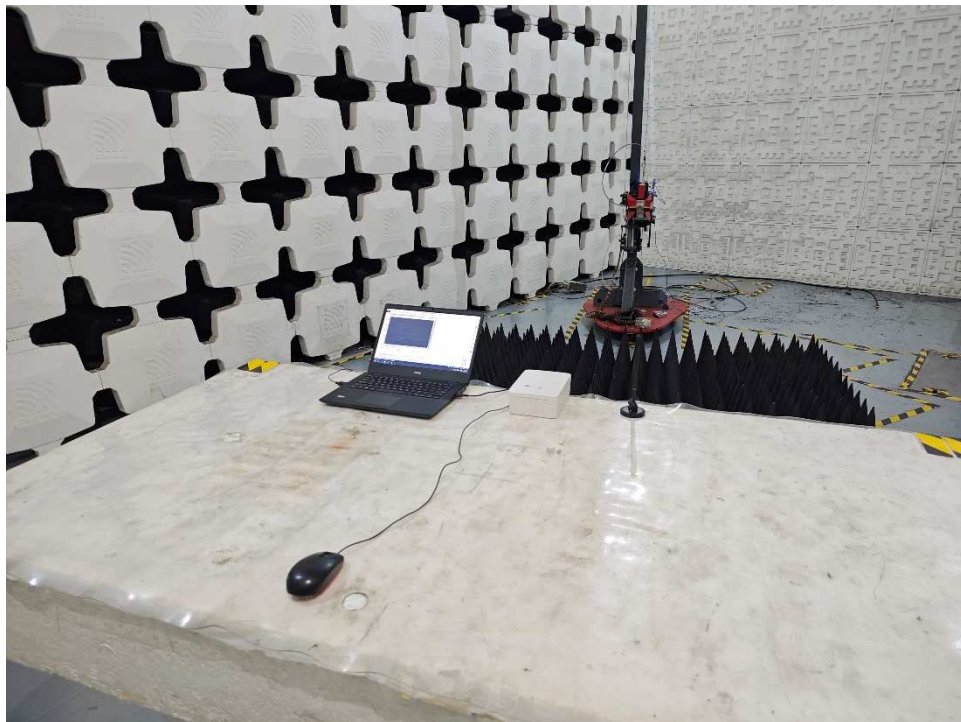
Photograph 2: Set-up for Radiated Emissions, above 1GHz
