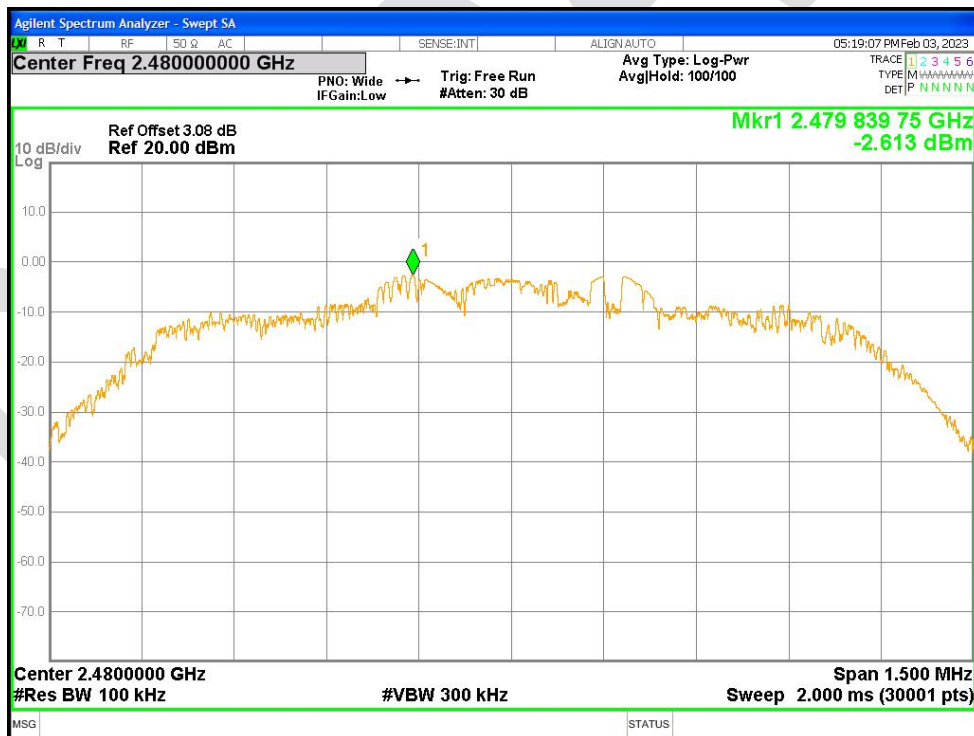
Tx. Spurious NVNT 3-DH1 2480MHz Ant1 Emission
