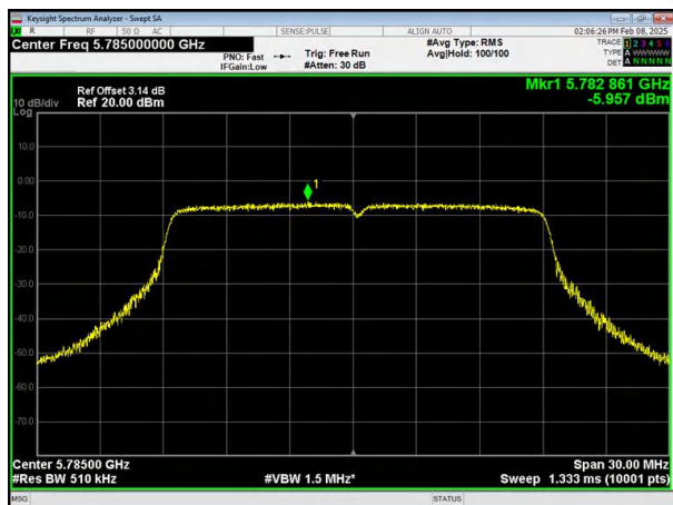
(802.11n20) PSD plot on channel 157
