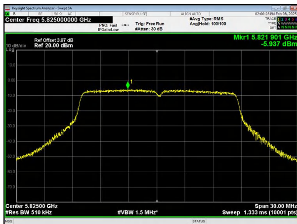
(802.11a) PSD plot on channel 165
