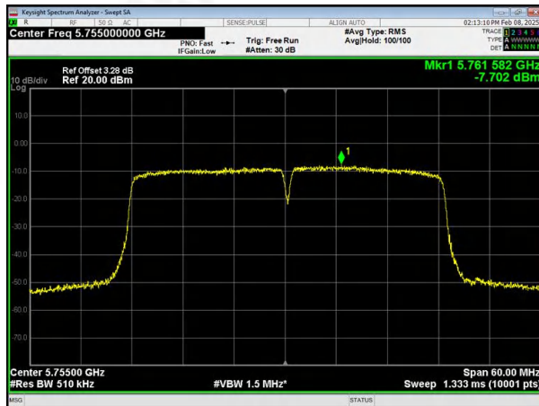
(802.11n40) PSD plot on channel 151
