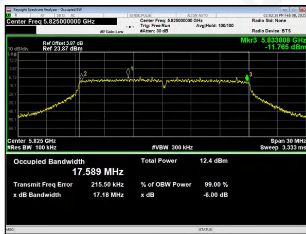
(802.11ac20) 6dB Bandwidth plot on channel 165
