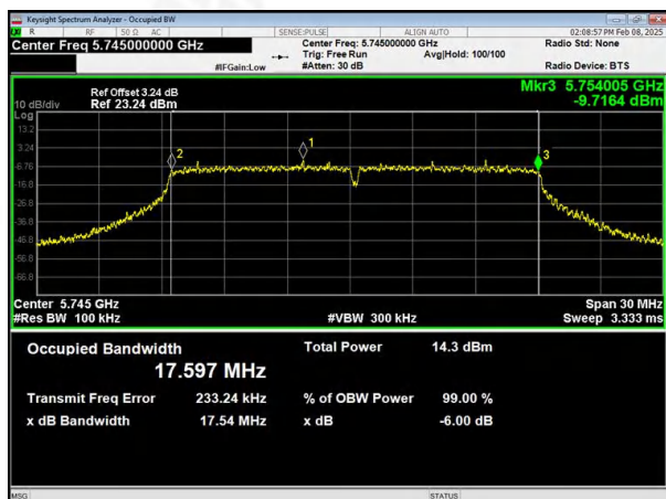
(802.11n20) 6dB Bandwidth plot on channel 149
