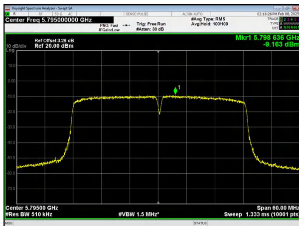
(802.11n40) PSD plot on channel 159
