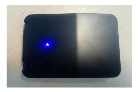
Note: When performing a site survey prior to installation, the BBM can be left in this mode to review the signal strength as you move around the build.
