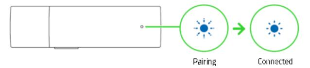
Once connected, the WIRELESS MICROPHONE will automatically reconnect to the last device whenever on and within range. Keep the devices within close proximity of each other for a faster and more stable connection.
