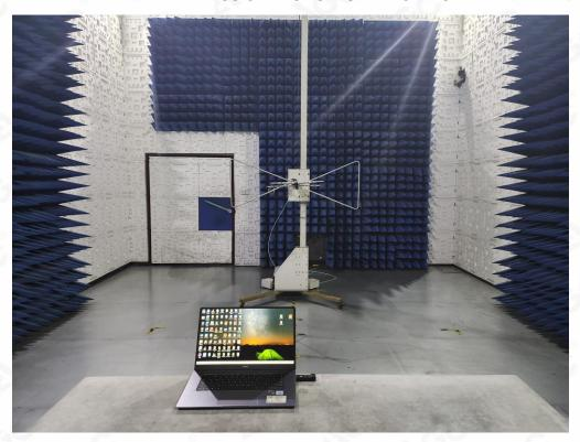
RADIATED EMISSION TEST SETUP ABOVE 1GHz
