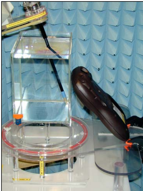
Figure 39. Positional photograph 4121GPRS at angle to phantom top facing
