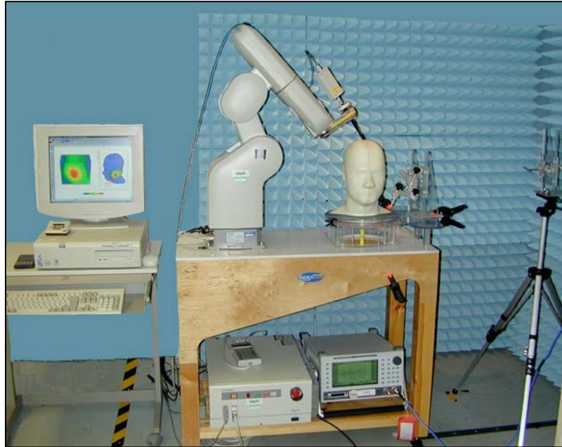
Figure 13: Principal components of the SAR measurement test bench
