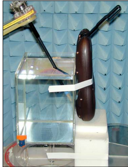
Figure 38. Positional photograph of 4121GPRS touch position rear facing
