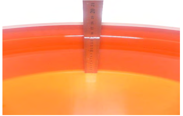
Photo 8: Tissue Simulant Liquid for Body 2450
