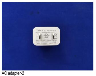
AC adapter-1: Model, KA06E-0501000US; Input:100-240V~50/60Hz, 0.25A Max;Output:5V DC, 1000mA; AC adapter-2: Model, TEKA006-0501000UK; Input: 100-240V~50/60Hz, 0.3A Max;Output:5V DC, 1000mA;
