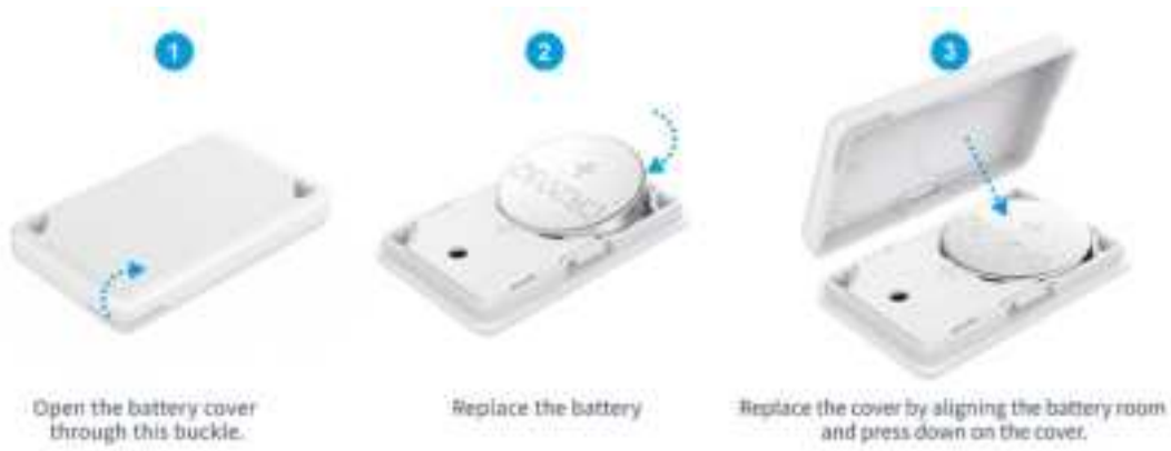
Figure 2: How to replace the battery of M4/M4S products?
