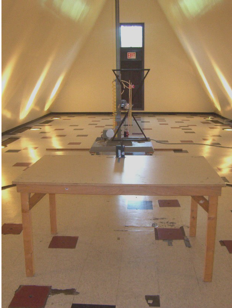
Radiated Emission Test Setup – Vertical Straight Up (Rear View)
