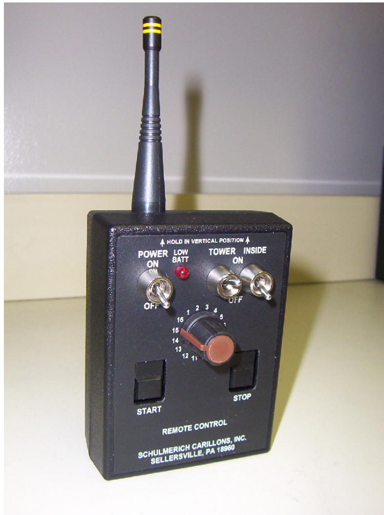
Photo 1 – Generation4 Outdoor Radio Remote Control – Front View
