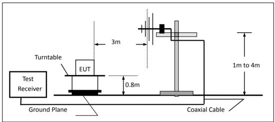
(c) For radiated emissions above 1000MHz
