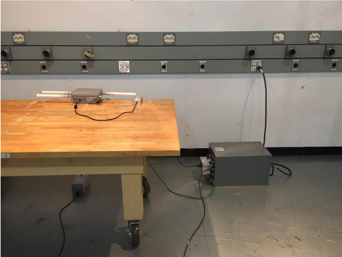
AC Mains Conducted Emissions setup
