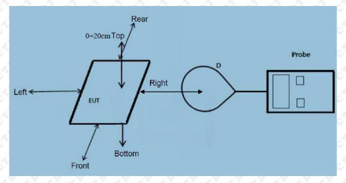
Note: Measurements should be made from all sides and the top of the primary/client pair, with the 20 cm-0cm measured from the center of the top, and 20cm-0cm measured from the center of the rest
