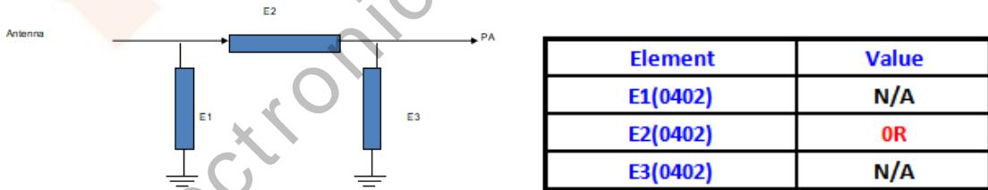
Schematic diagram of matching circuit modification
