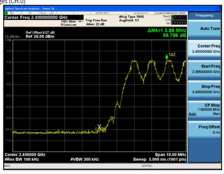
Test Plots with hopping (GFSK)
