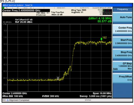
Test Plots with hopping ( $\pi/4DQPSK$ )
