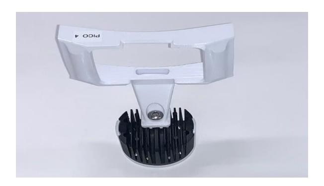
2. Snap the plastic bracket in place on the HMD host
