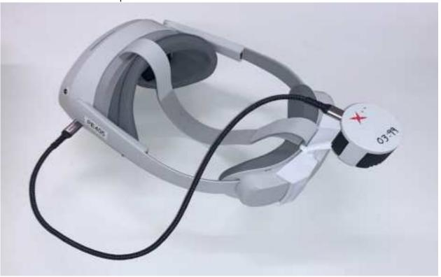
4. To charge the Host, disconnect the USB-C cable to the module and use the supplied OEM charger and charging cable.
