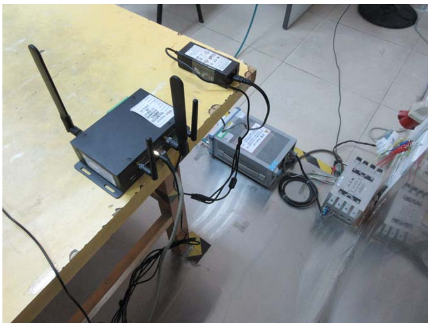
Conducted Emissions Test Setup – Side View (for Adapter 3)
