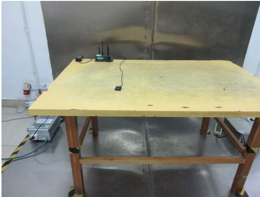
Conducted Emissions Test Setup – Front View (for Adapter 2)
