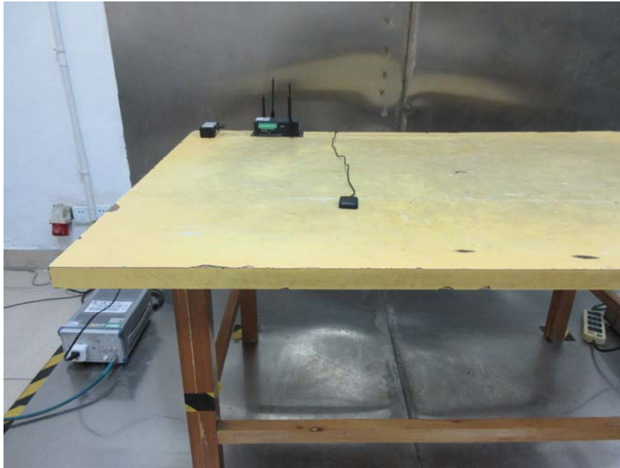
Conducted Emissions Test Setup – Front View (for Adapter 3)
