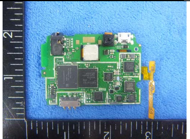
Mainboard Without Shielding - Front View
