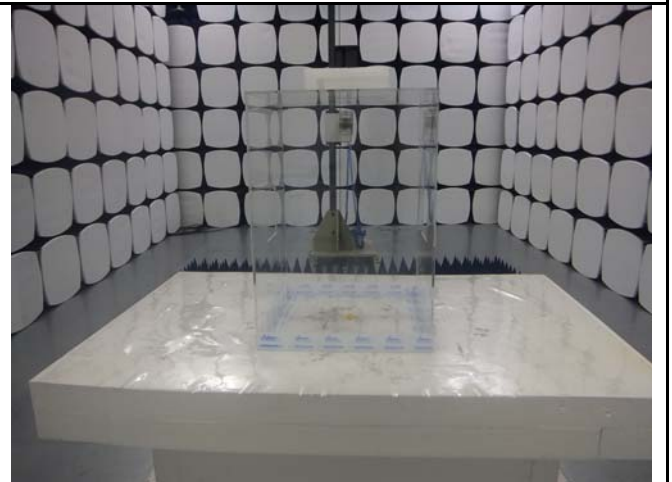
Radiated Spurious Emissions Test Setup Above 1GHz
