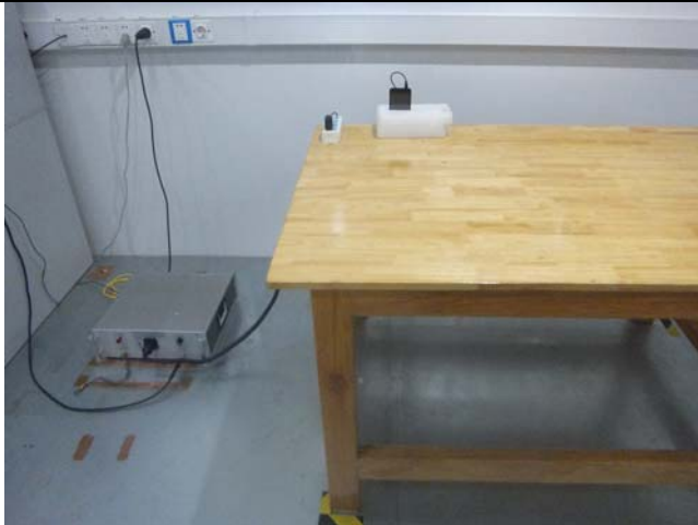
Conducted Emissions Test Setup Front View
