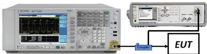
Figure 7-4. Test Instrument & Measurement Setup
