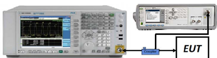
Figure 7-5. Test Instrument & Measurement Setup
