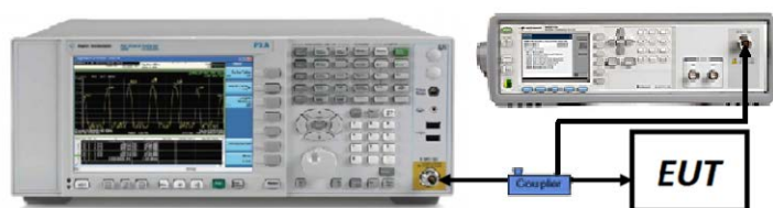
Figure 7-6. Test Instrument & Measurement Setup
