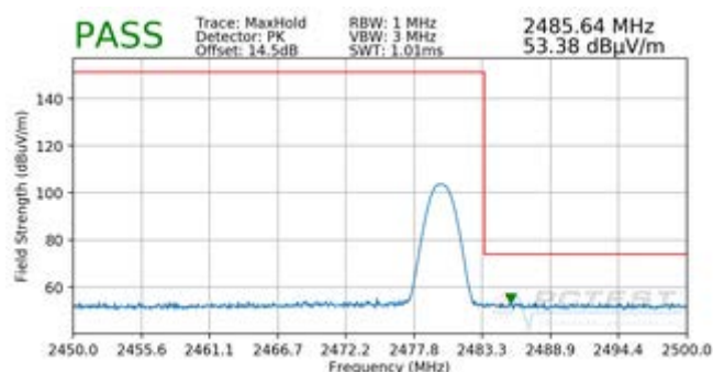
Plot 7-47. Radiated Restricted Upper Band Edge Measurement (Peak)
