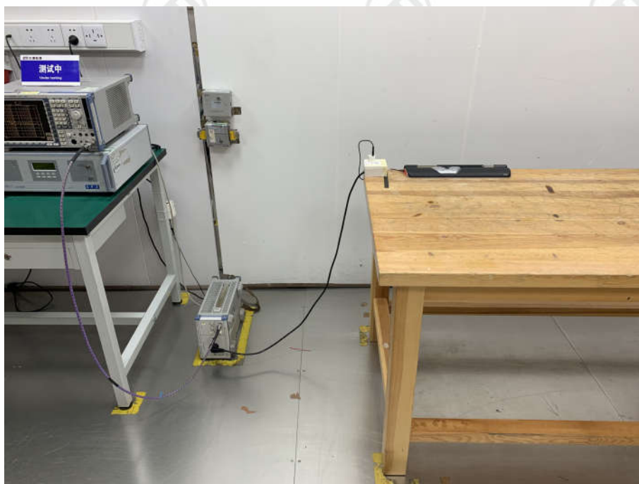
Conducted Emissions Test Setup
