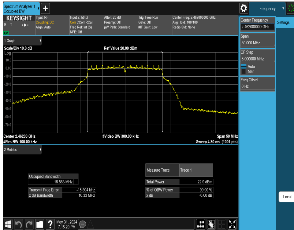
Plot 7-33. 6 dB BW and 99% OBW Plot Antenna WF7 (802.11g – Ch. 11) – 12Mbps
