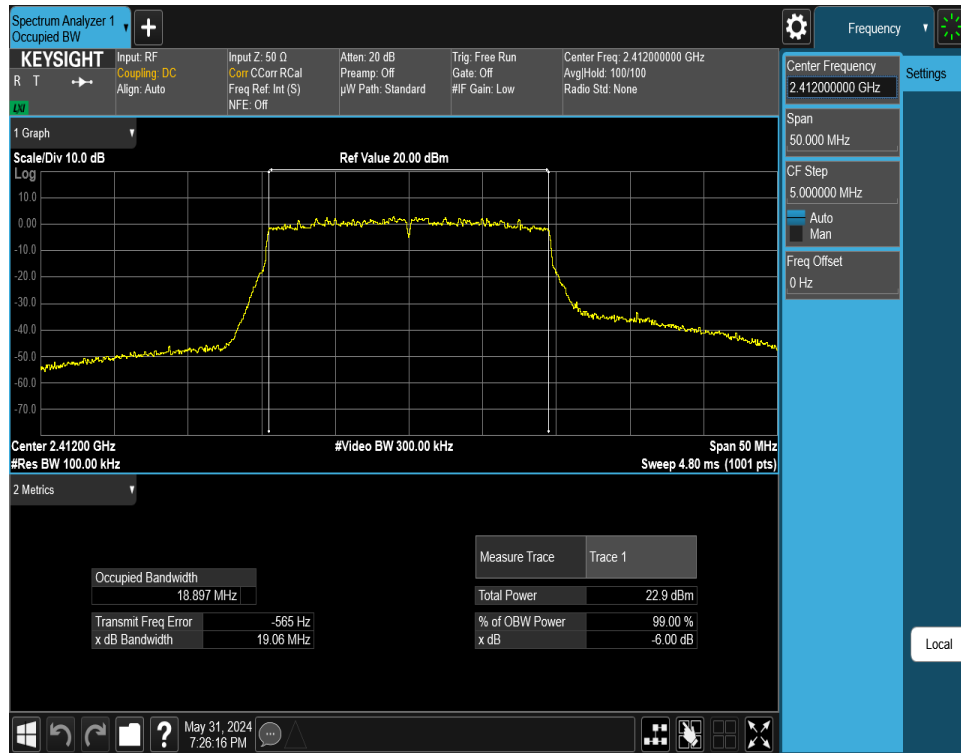
Plot 7-46. 6 dB BW and 99% OBW Plot Antenna WF7 (802.11ax (SU - 2.4GHz) – Ch. 1) – MCS4
