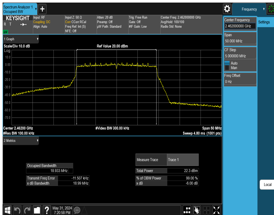
Plot 7-39. 6 dB BW and 99% OBW Plot Antenna WF7 (802.11ax (SU - 2.4GHz) – Ch. 11) – MCS2
