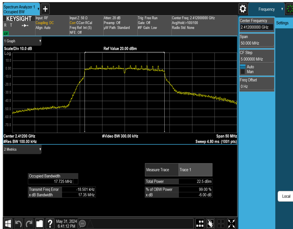
Plot 7-4. 6 dB BW and 99% OBW Plot Antenna WF8 (802.11n (2.4GHz) – Ch. 1) – MCS2
