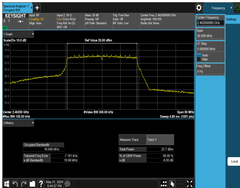
Plot 7-9. 6 dB BW and 99% OBW Plot Antenna WF8 (802.11ax (SU - 2.4GHz) – Ch. 11) – MCS2
