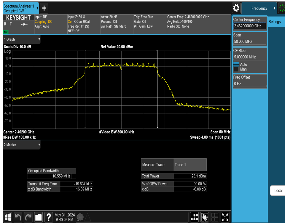
Plot 7-3. 6 dB BW and 99% OBW Plot Antenna WF8 (802.11g – Ch. 11) – 12Mbps
