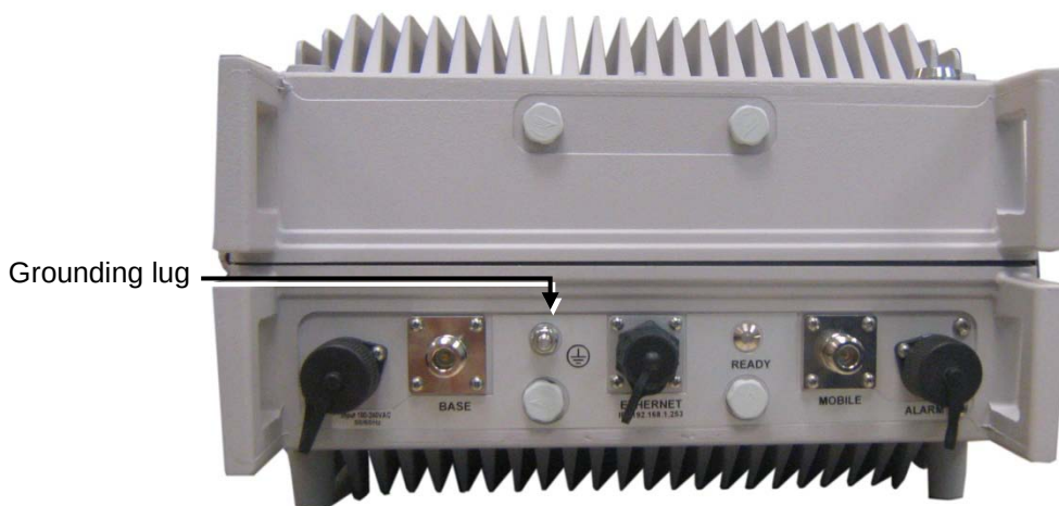
Figure 3-1. D-SBR Repeater Grounding Lug
