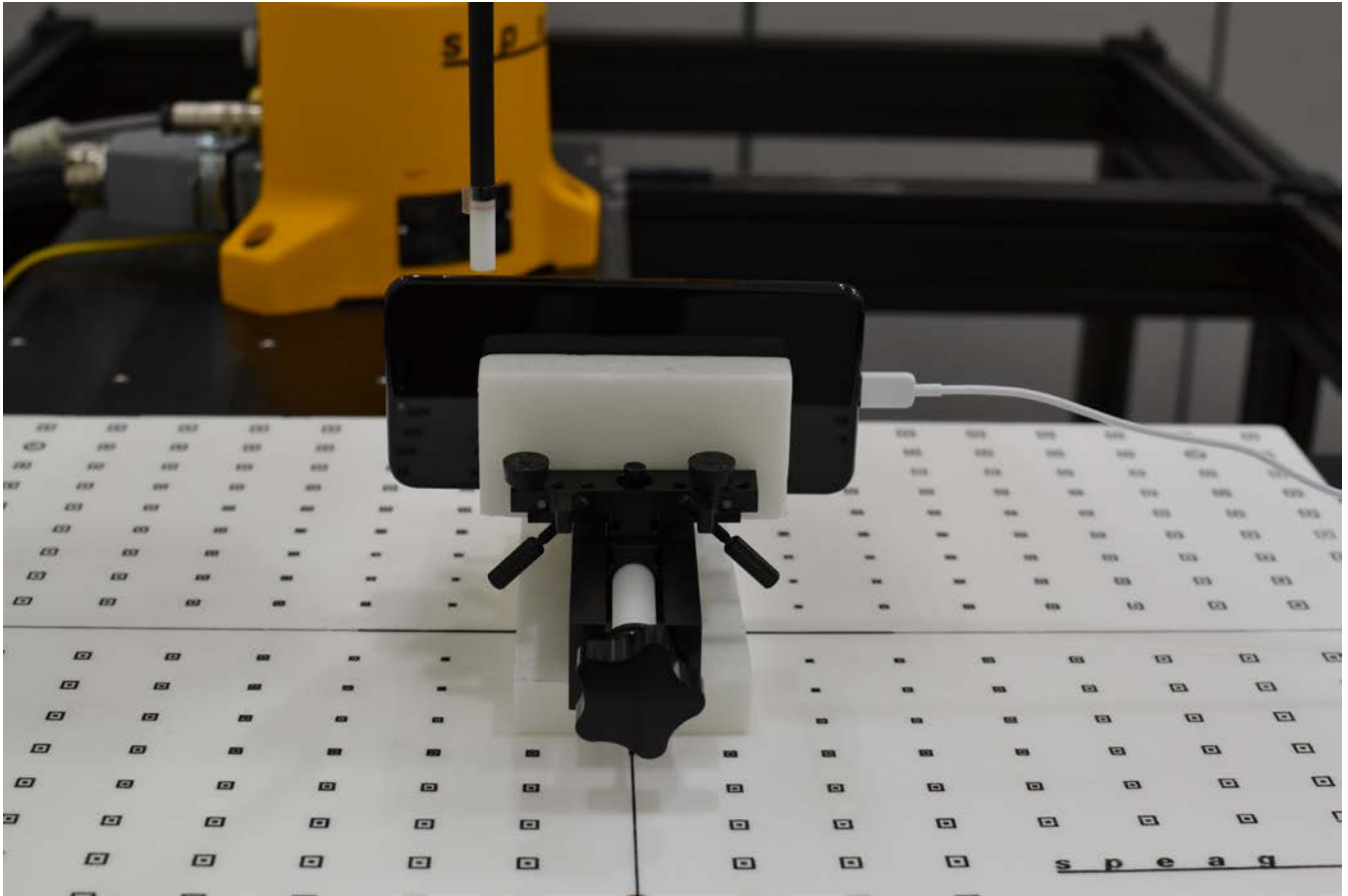
Near-Field Power Density Test Setup Photo 3 – Right Edge at 2mm
