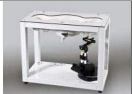
Fig. 6.8 Photo of SAM Phantom
