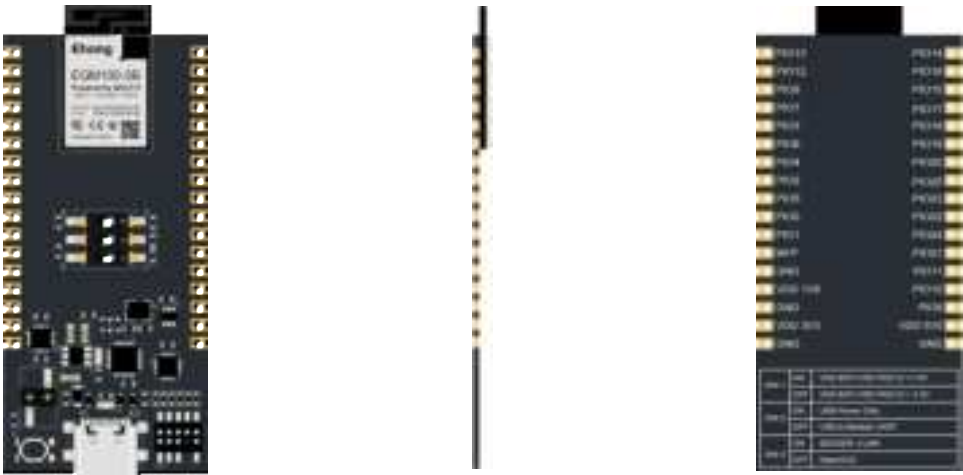
Figure 4: EQM100-5B Module Development Kit
