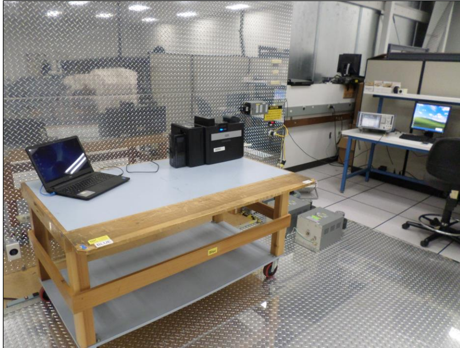
Photograph 1. Conducted Emissions, Station Setup
