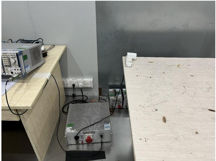
Conducted Emission Test Setup
