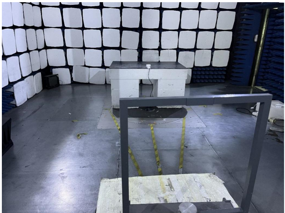
Radiation Emission Test Setup (Below 30MHz)
