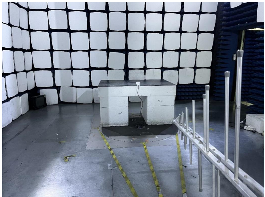
Radiation Emission Test Setup (30MHz to 1GHz)
