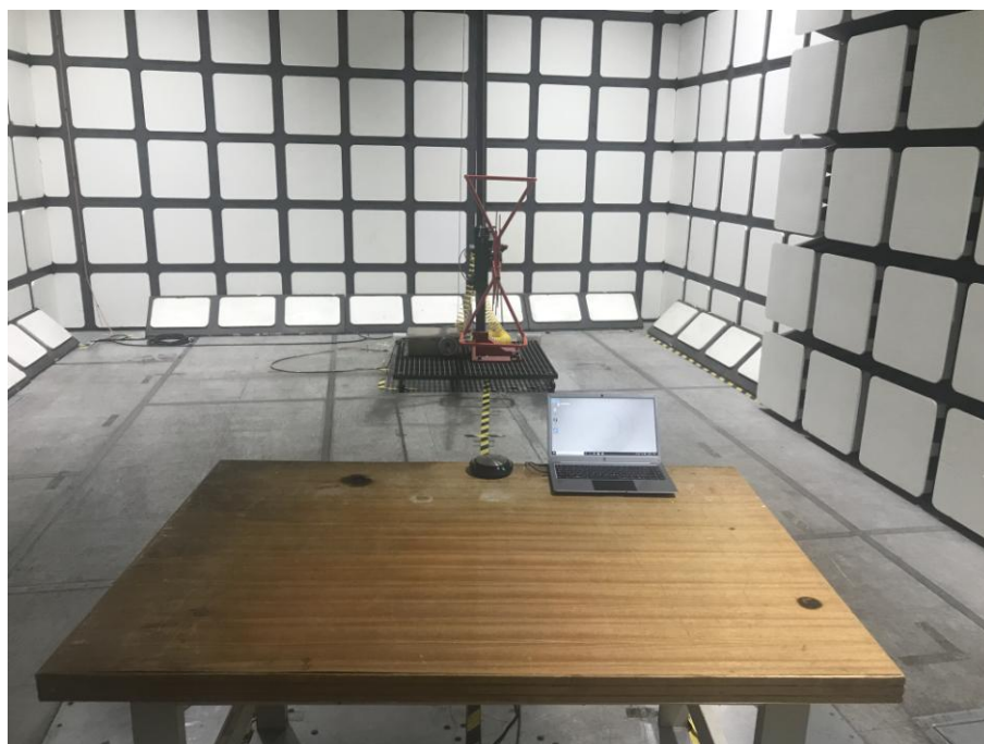
Radiated Emissions – Front View (Below 1 GHz)
