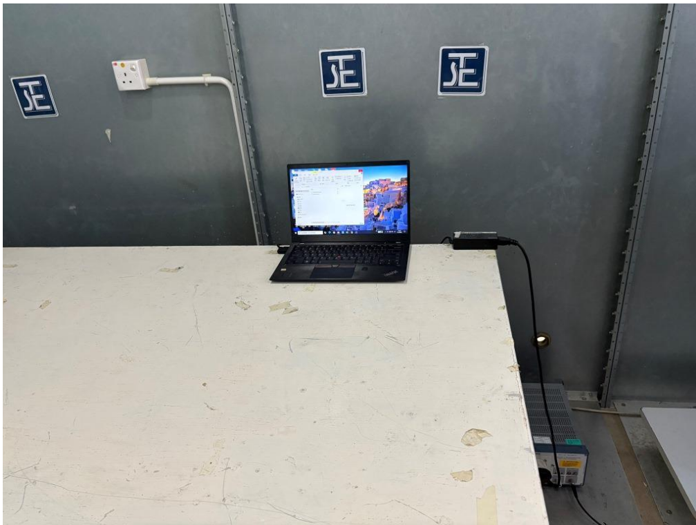
Measurement of Conducted Emission Test Set Up
