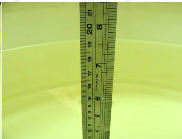
Photo of Liquid Height for Body SAR
