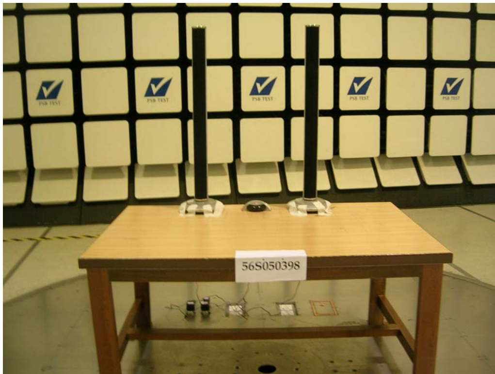
Radiated Emissions Setup (Front View)
