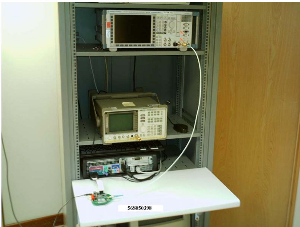
Maximum Peak Power Measurement Test Setup
