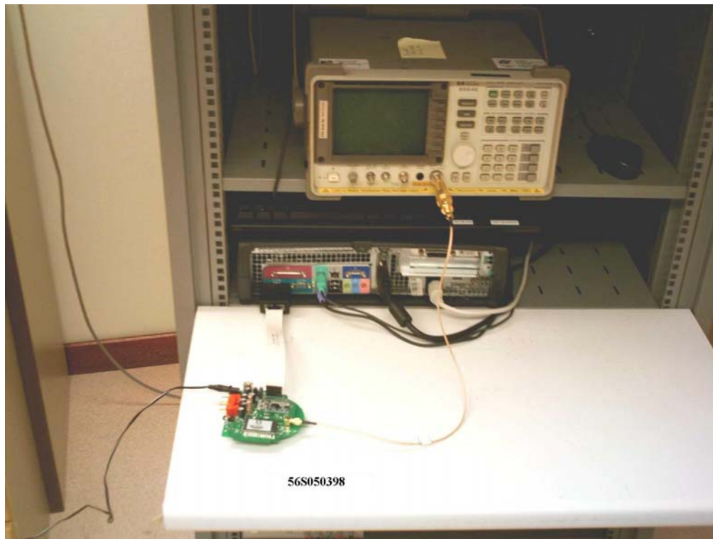
Average Frequency Dwell Time Measurement Test Setup
