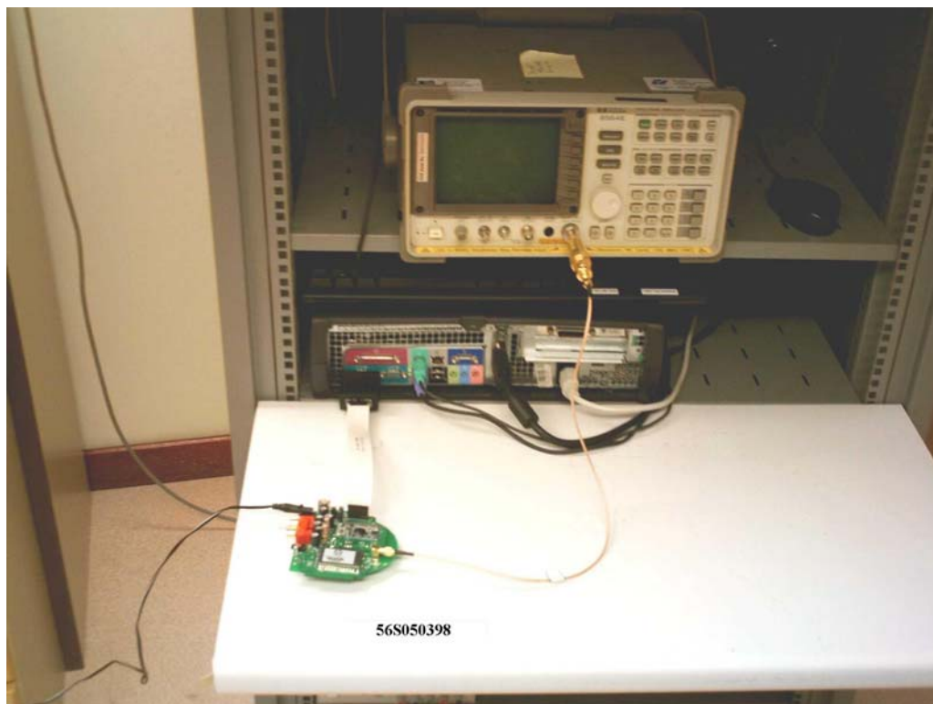
Number of Hopping Frequencies Measurement Test Setup
