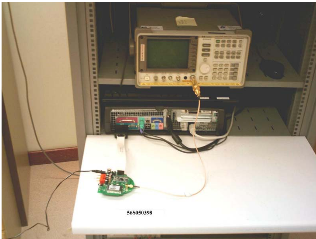
Peak Power Spectral Density Measurement Test Setup
