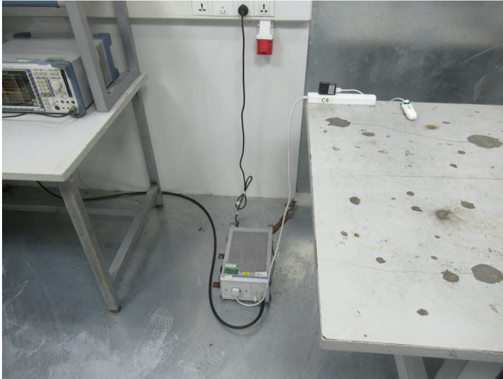
Photo of Conducted Emission Measurement
