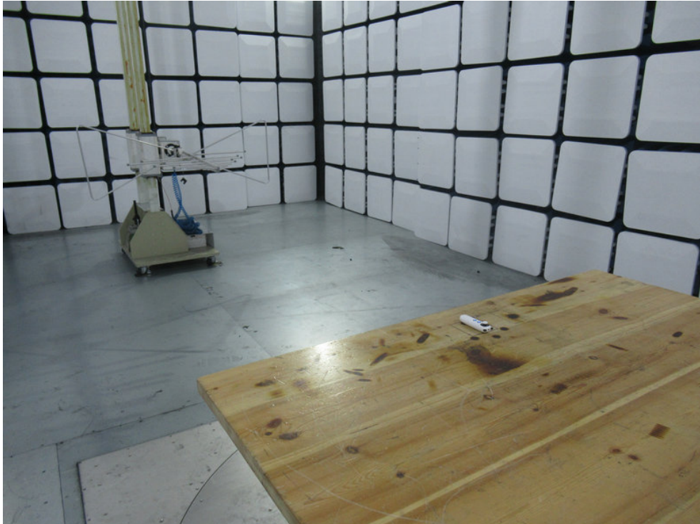
Photo of Radiation Emission Test
