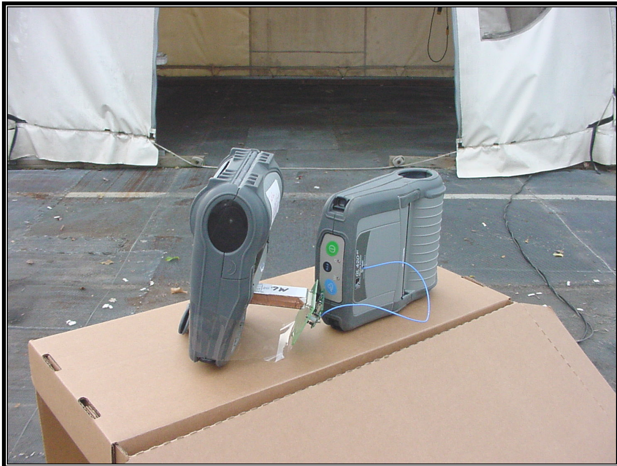
PHOTOGRAPH 2: RADIATED EMISSION FRONT VIEW; WORST CASE CONFIGURATION RW-420 (CQ17109-1) ANTENNA
