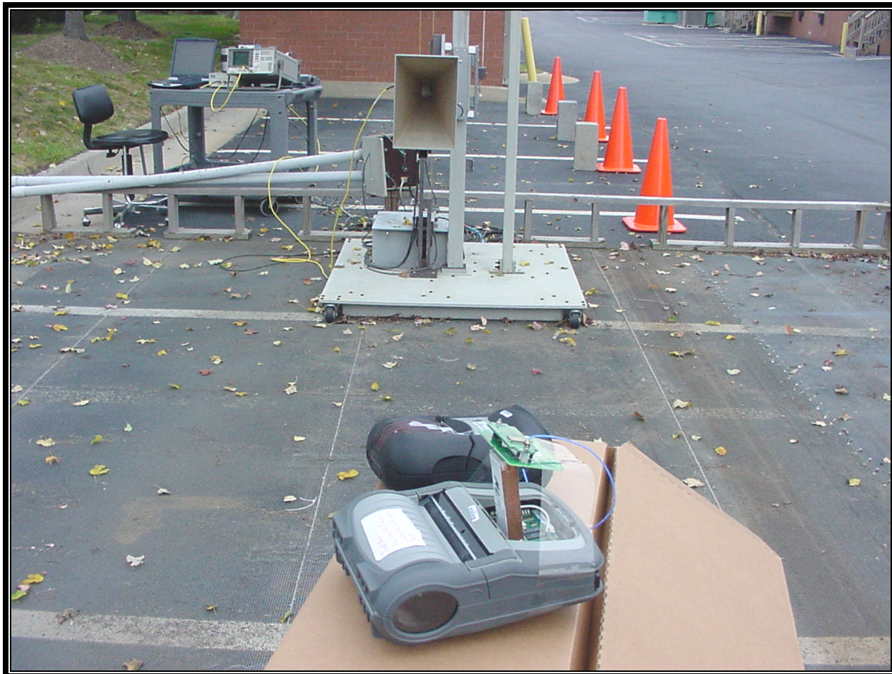
PHOTOGRAPH 3: RADIATED EMISSION REAR VIEW; WORST CASE CONFIGURATION RW-420 (CQ17109-1) ANTENNA
