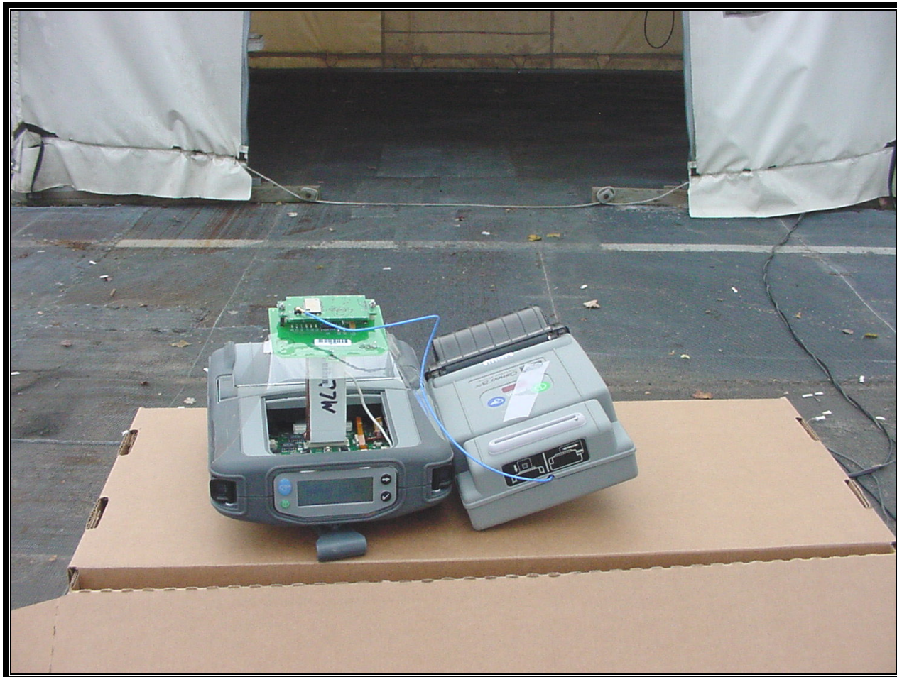
PHOTOGRAPH 4: RADIATED EMISSION FRONT VIEW; WORST CASE CONFIGURATION CAMEO 3 SC (CQ16142-1) ANTENNA
