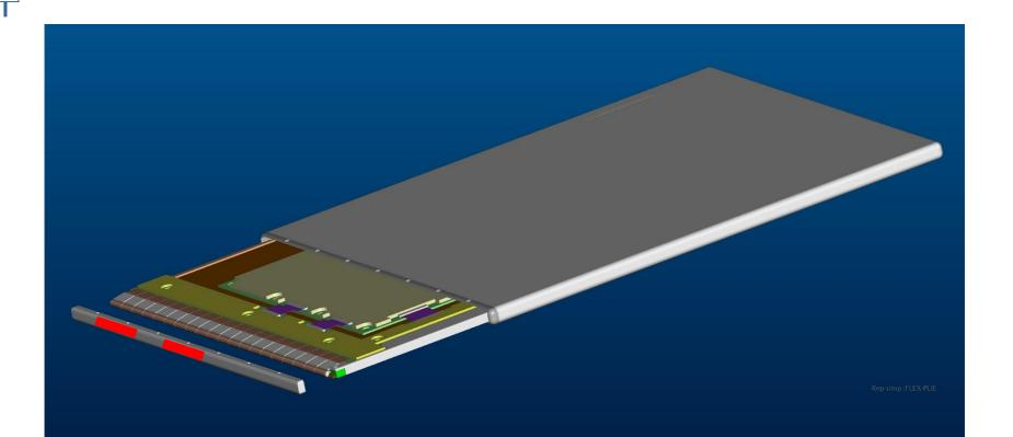
The same mechanical concept is used for the three detectors. The antennas are located on the cap (in red on the drawing). The cap is screwed to the housing.
