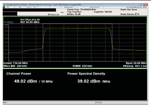
Port 1, Band n12, 729 - 745 Mhz, 10 MHz Bandwidth, 256QAM Modulation, Mid Channel, 737.0 MHz
