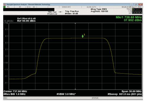
Port 1, 5G NR, Band n12, 729 - 745 Mhz, 15 MHz Bandwidth, 256QAM Modulation, High Channel, 737.5 MHz
